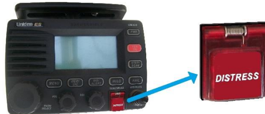
DSC Radio Distress Button
