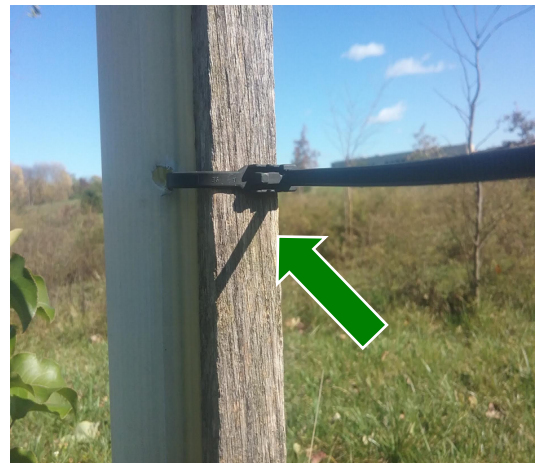
Arrow showing easy push-release button on zip ties, which can be reused by landowners
