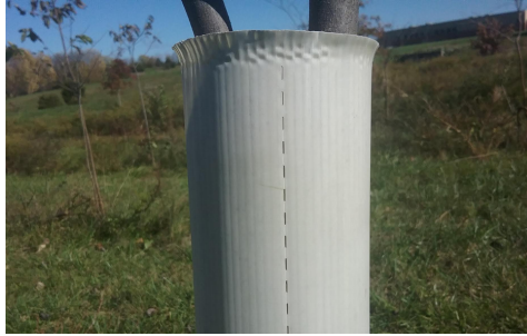
Corrugated seam of shelter (left), shelter on 6-year-old tree breaking off along seam (right)
