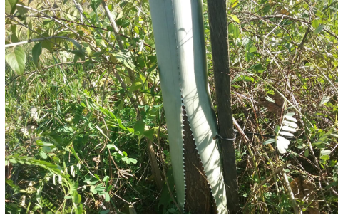
Corrugated seam of shelter (left), shelter on 6-year-old tree breaking off along seam (right)
