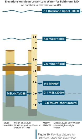
Figure 10. Key tidal datums for Baltimore. Minor and major flood levels are based on a nationally consistent approach; thus the minor flood level is higher than previously used to define nuisance flooding.
