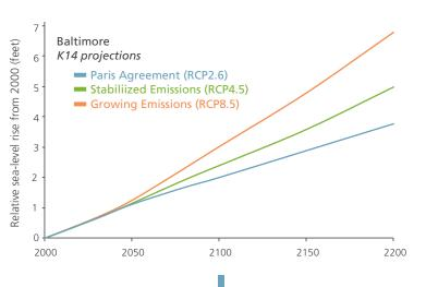
Figure 7. Median projections of relative sea-level rise at Baltimore through 2200 under the three greenhouse gas emissions pathways.
