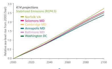
Figure 6. Median projections of sea-level rise at several tide-gauge locations in the Chesapeake Bay through 2100. Differences are attributable to different rates of vertical land motion.
