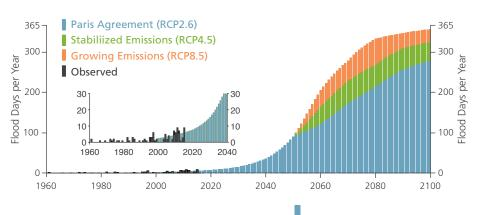
levels would exceed this minor flood threshold based on the 2018 sea-level rise projections included in this report. Note that this is based on the recently derived, nationally consistent threshold for minor flooding,<sup>33</sup> not the lower NOAA flood threshold represented in Figure 1.
