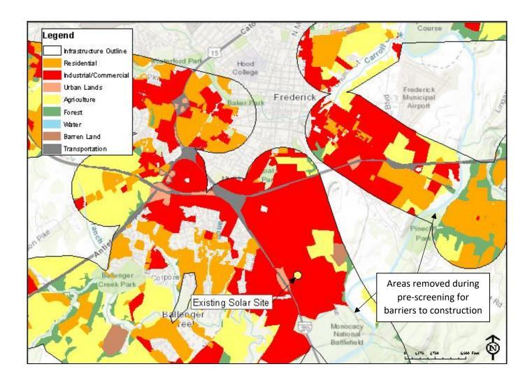
SmartDG+ screens out areas that have potential barriers to construction and therefor might be unsuitable for siting solar or wind projects. The image above shows a 1 mile corridor around 3-phase <= 35kV distribution lines with land use / land cover that remains after the screens are applied.
